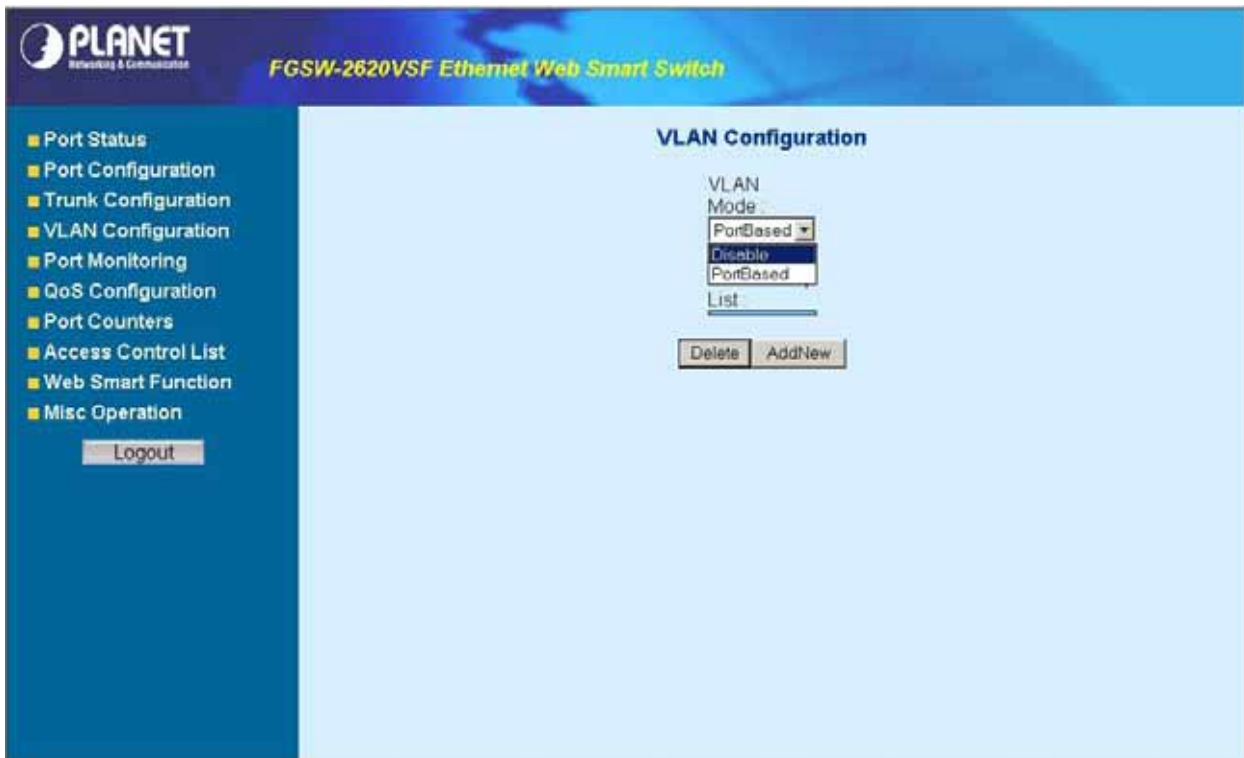
Figure 4-23 Disable Port-based VLAN function Web Page screen
